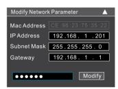
For example, if the IP address of your computer is 192.168.1.4, then you will need to modify the IP address of the camera to 192.168.1.x. After modifying, please enter the password of the administrator and click the "Modify" button to modify the IP settings.
