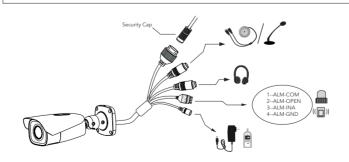
\*1 It is recommended to install the security cap for outdoor installation.
